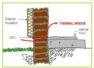
Between floors: if insulating internally, the insulation will need to stop at the ground floor ceiling level and continue from first floor level. To avoid a thermal bridge between the floors, insulation between floor joists at the junction with the external wall can be added.
