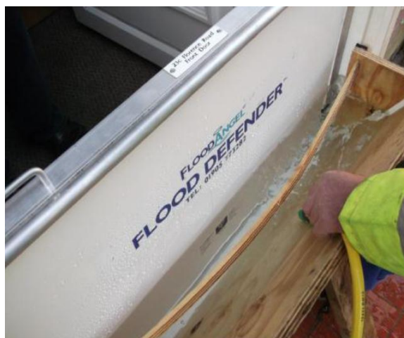
Example of a flood barrier being tested (source Defra report FD2668)
