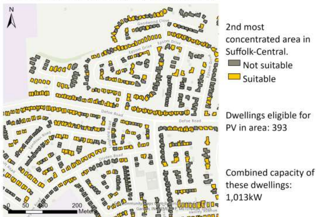
Figure 67: Dwellings identified as suitable for rooftop PV panels. (Location: Whitton, Ipswich )
