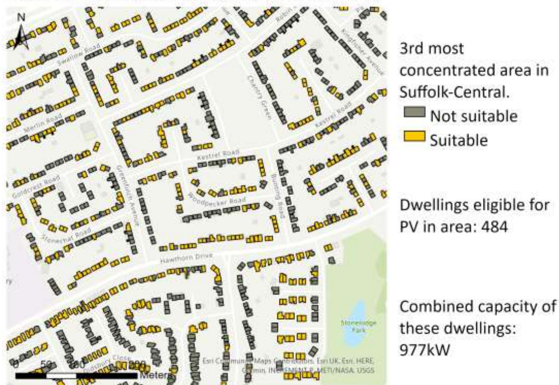
Figure 68: Dwellings identified as suitable for rooftop PV panels. (Location: Chantry, Ipswich )
